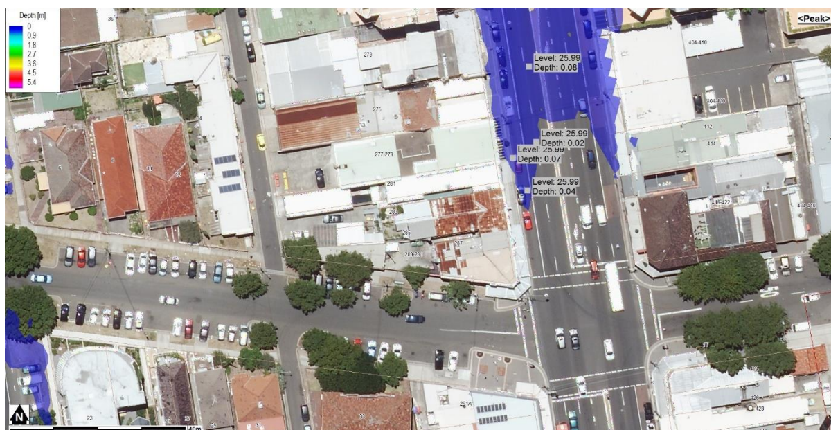
Figure 1- Flood Levels & Depths 1% AEP (1 in 100yr) flood
